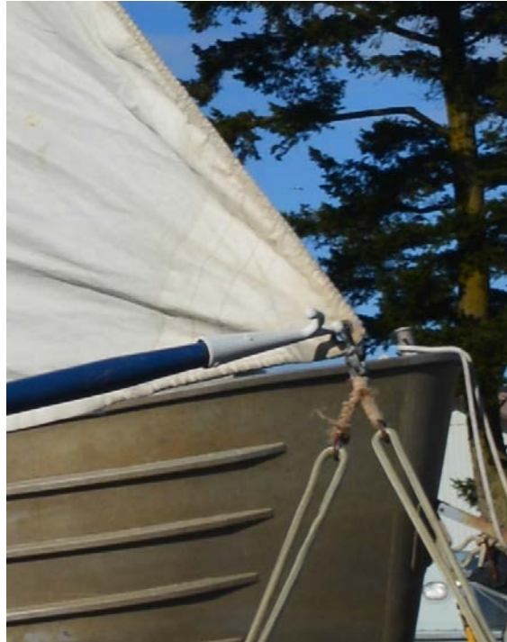
Bullseyes with whips roved through
