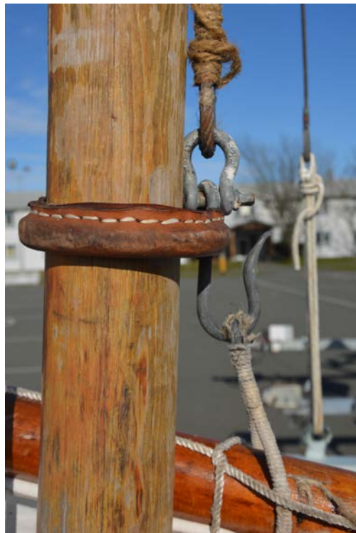
Yard hooked into traveler
