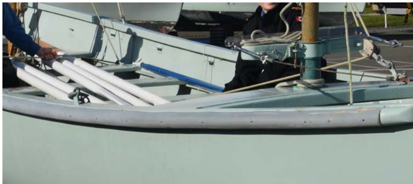
Eyeplates, sternsheets, and standing blocks
