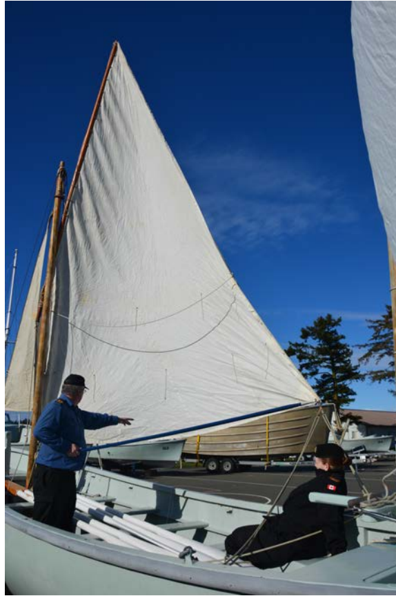
Brail and Spreader/Bearing out Spar being used on foot of mainsail
