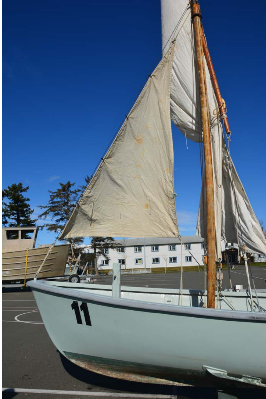
Foresheets, clip-hooks, and the clew of the foresail
