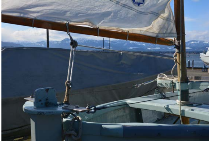
Mizzensheet from boom through block/deadeye on stern post
